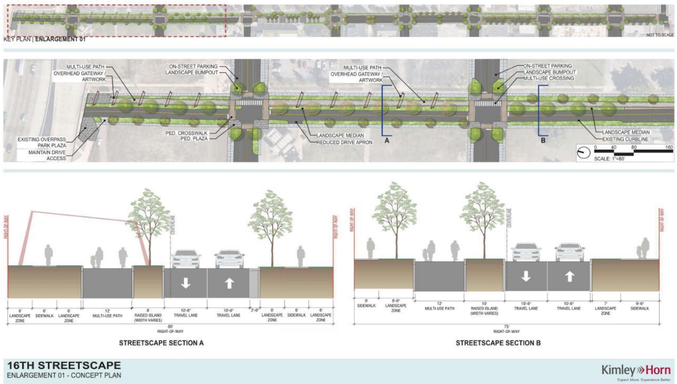
Figure 9 – Typical Section 1 (City Walk to 6th Ave)
