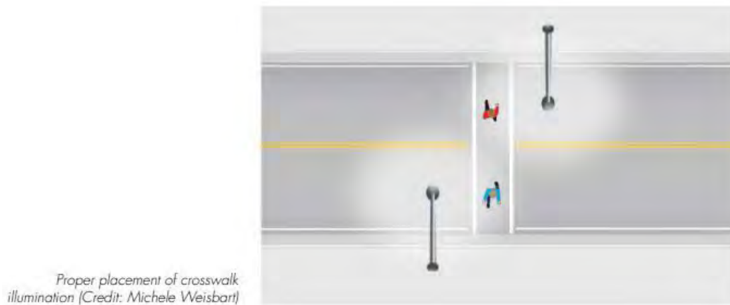
Figure B-14: Lighting at a Crosswalk (Source: PEDSAFE)
