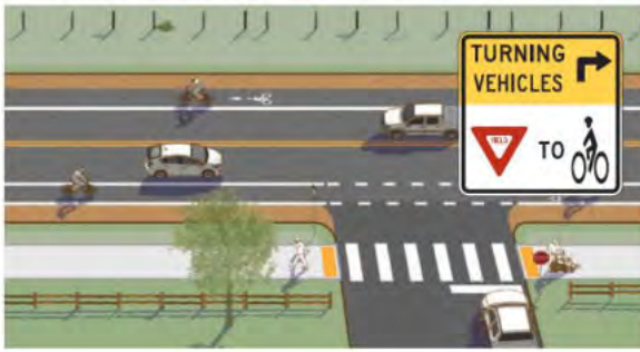
Figure B-16: Proper bicycle lane striping at a side street intersection (Source: FHWA)
