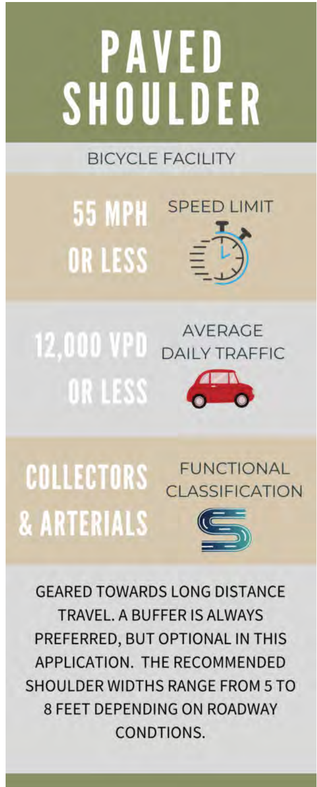
Figure B-10: Paved Shoulder Guidance
