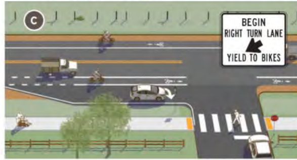
Figure B-16: Proper bicycle lane striping at a side street intersection (Source: FHWA)
