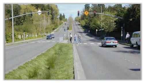
Figure 21: Pedestrian Hybrid Beacon Example (Source: FHWA)
