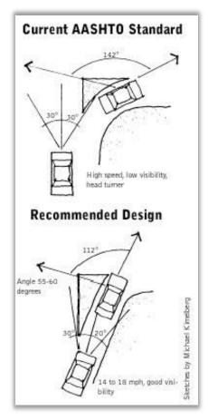
Figure 22: Smart Channel Right Turn Lane Geometry (Source: FHWA)
