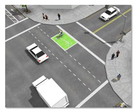
Figure 10: Two-Stage Left Turn Queue Box (Source: NACTO)
