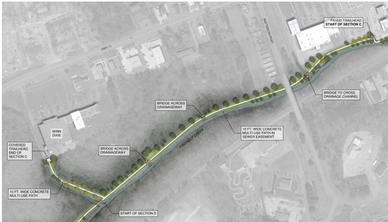
Figure 12: Section C Conceptual Diagram of Proposed Improvements
